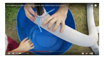
9. Coil the 7 foot drainage tube in the bottom of the barrel making sure to keep an empty place in the center.
