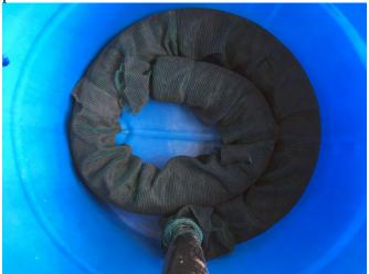
10. Secure top of water feeder tube to top of barrel.
